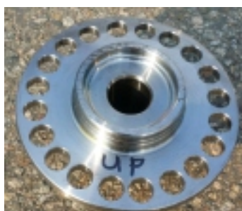
After drilling & front chamfering
