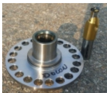
After drilling & back chamfering
